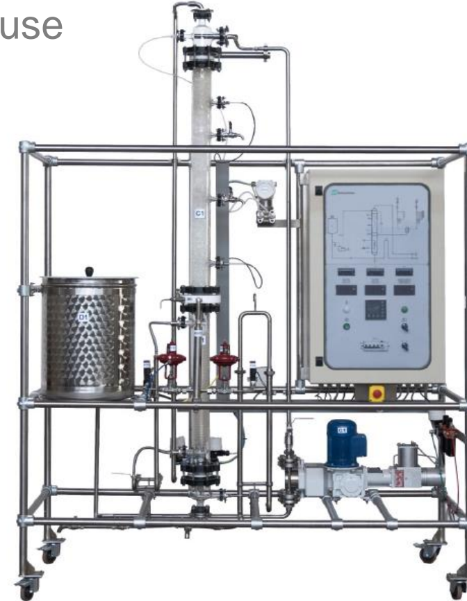
1m (80mm ID) packed column (Raschig rings)
