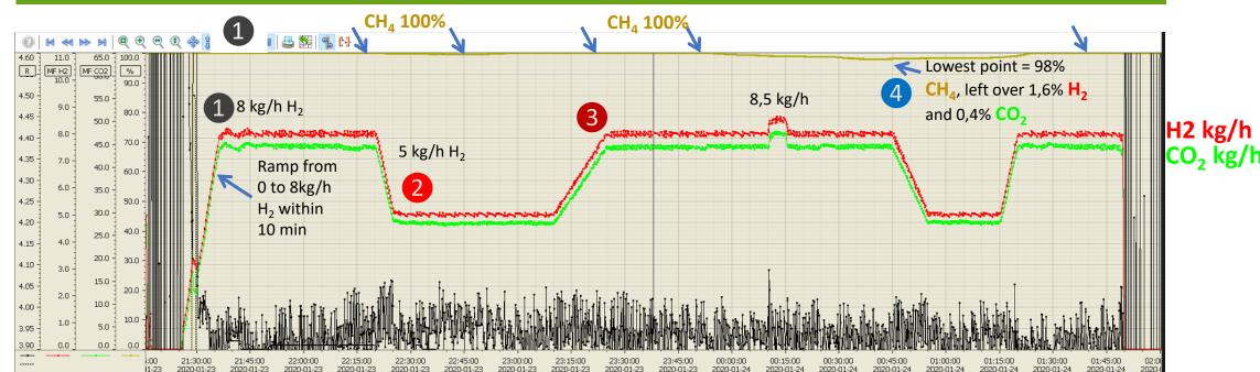
Start-up within minutes, CH<sub>4</sub> production achieves designed scale of the test performed
